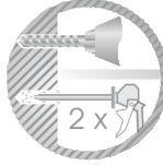
Drill the hole (see technical data). Blow out the dust with compressed air (>6 bar) twice.
